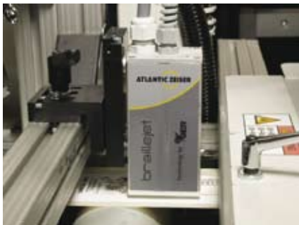
The Braillejet print head prints two lines of Braille simultaneously
