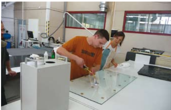
Figure 5: Manual cleaning and pre-treatment at a customer's site
