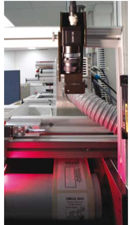
Braille Vision's inline camera provides complete quality control of the production processes
