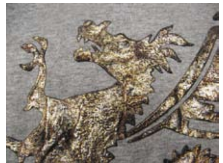
Multiple foil application showing adhesion properties of plastisol
