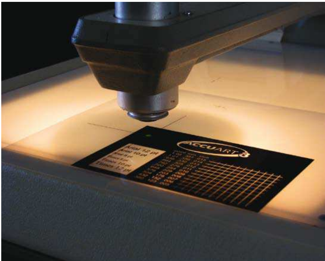
Testing D_{max} value, a measure of print density, using a densitometer
