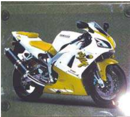
Figure 9: Print with CMYK + white ink on glass, then laminated as safety glass [4]
