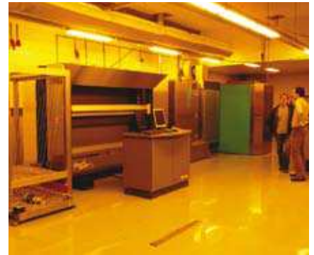
In-Line with CtS system, automatic developing, de-stacking and final drying
