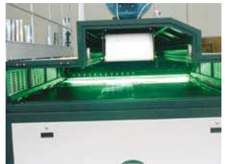
The electronically-controlled UV plus reflector rotates 180 degrees
