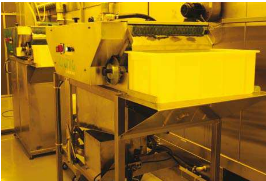
The G-Wash 040 In-House water preparation and solvent cleaning system uses an inclined filter
