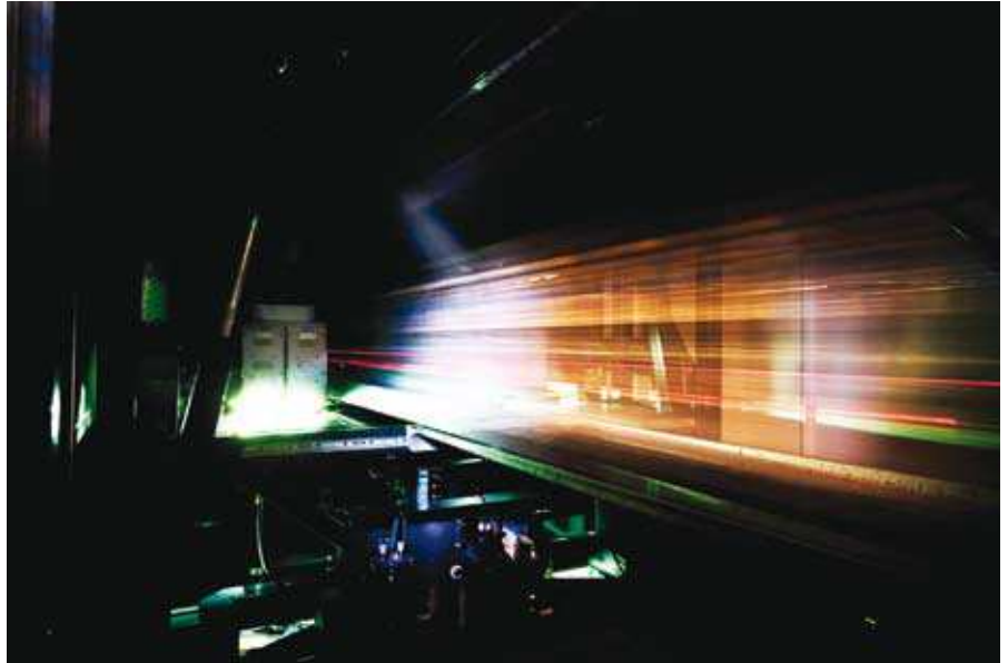
Onset is equipped with 576 printheads arranged across the width of the print bed
