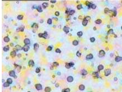
Figure 2: Poor drying and unfavourable wetting cause individual drops to bleed and develop into unfilled oval dots
