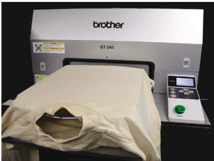
Figure 9: The Brother GT 541 is among the many direct-to-garment inkjet printers being used to produce full-colour photographic images on garments
