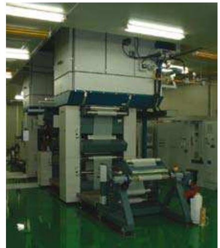
A rotary screen printing press prints RFID antennas in one pass
