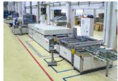
The tri-colour line is for the printing of flat glass for white goods
