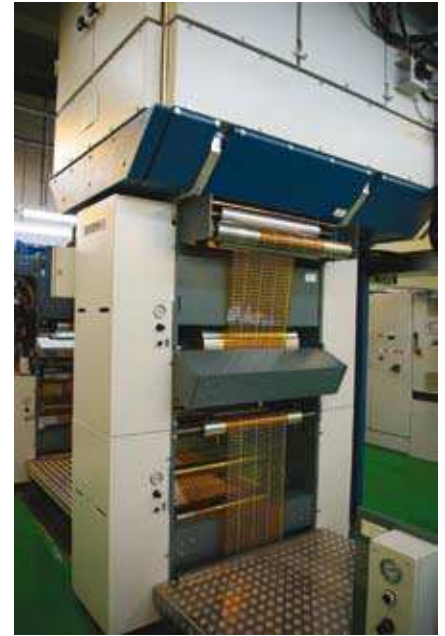
A rotary screen printing unit to print silver conductive ink for reel-to-reel antenna production
