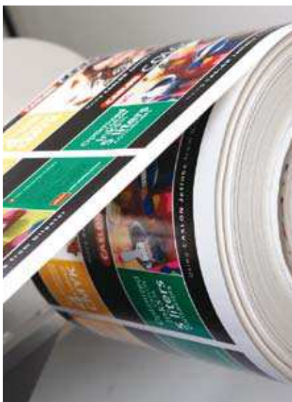
A Caslon label reel printed using the Nilpeter printer with Xaar 1001 printheads
