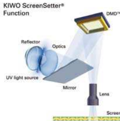
Figure 1: The principle of the light path of a DMD system using the KiWo ScreenSetter as an example
