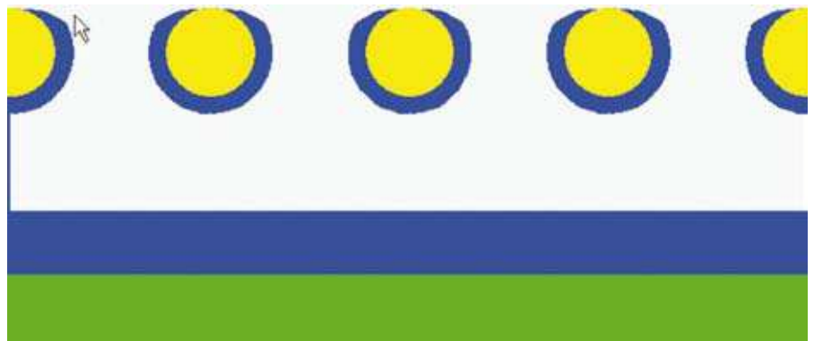
Ink deposit = Ink-in-the-mesh-at-the-start minus Ink-on-the-mesh-at-the-end
