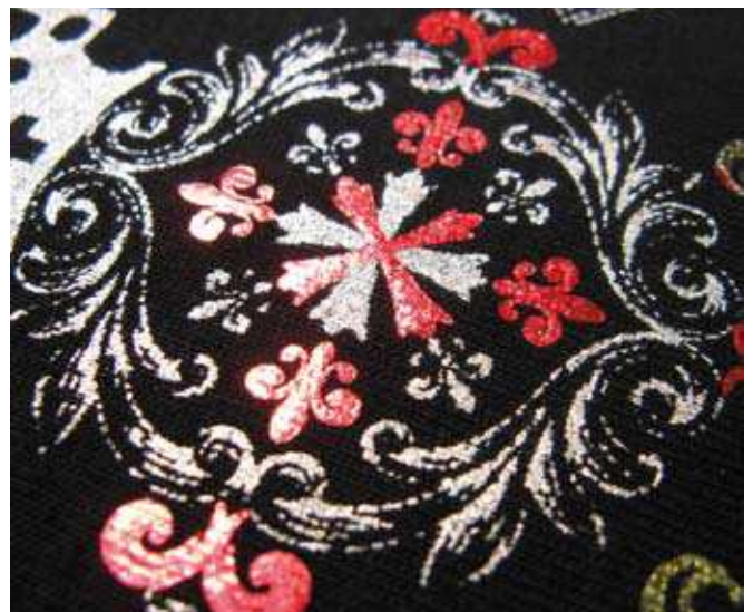
Figure 6: Solutions to the oxidation of metallic pigments include a clear coat and advising the consumer to hand-wash the garment
