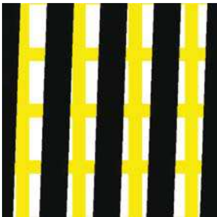
Thin mesh good, thick mesh bad for printing fine lines
