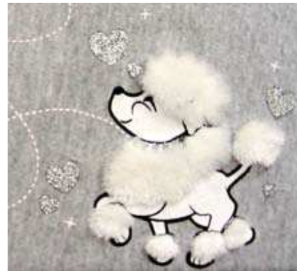
Figures 1 and 2: Because screen printing for garments is a low resolution application, a larger flake is used
