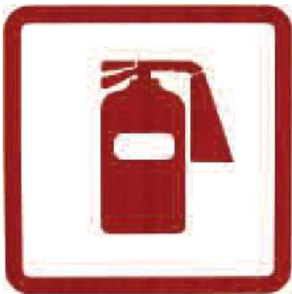
Fire extinguishers should be located within 75 feet (23 metres) of an exit and should be inspected every 12 months
