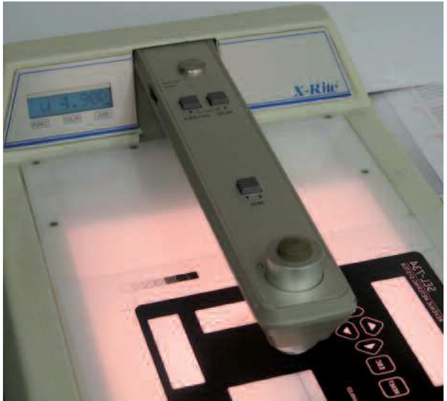
Figure 3: densitometer reading 4.9 UV opacity
