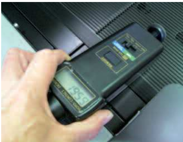
A handheld tachometer for confirming belt speeds
