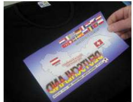
The design (printed in mirror image) has to be placed on the textile upside down (process using Subli-Dark Soft 501)
