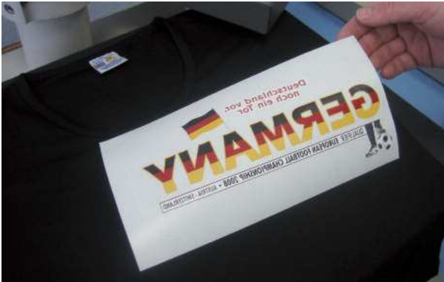
After printing (mirror image) and weeding (process using Subli-Dark 201)
