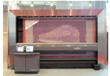
Large format CtS StencilMaster with standard 1270 dpi exposure resolution
