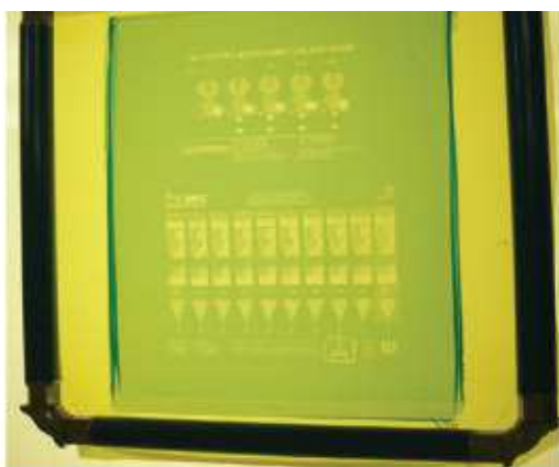
EVALUATION MUST BE DONE WHILE THE SCREEN IS WET TO PROPERLY SEE THE COLOR CHANGE.
