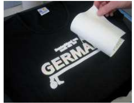
After 8 seconds the backing paper has to be taken off (process using Subli-Dark 201)
