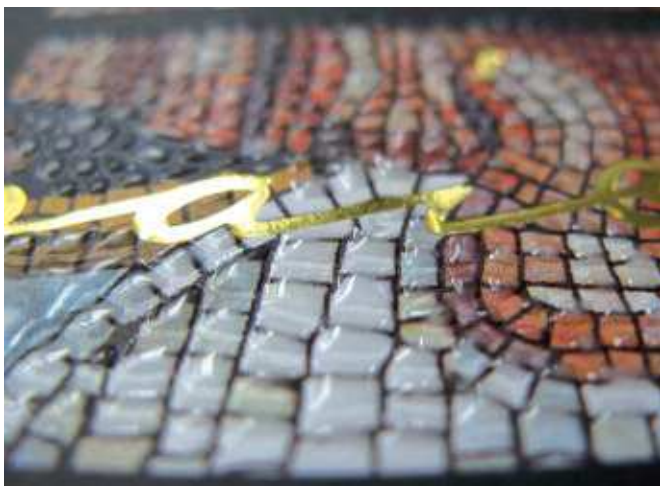
Tactile varnish on pre-printed HP indigo label (Franchini & Speri flatbed label)
