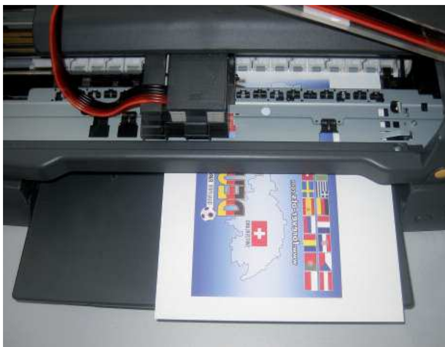
How it comes out of the printer (process using Subli-Dark Soft 501)
