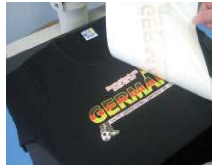
After the transfer process, the backing paper has to be taken off after about 10 seconds (process using Subli-Dark Soft 501)
