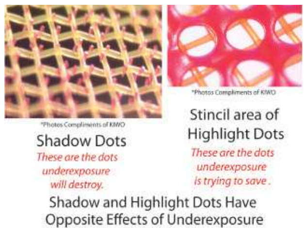
Figure 5: Opposite effects of underexposure
