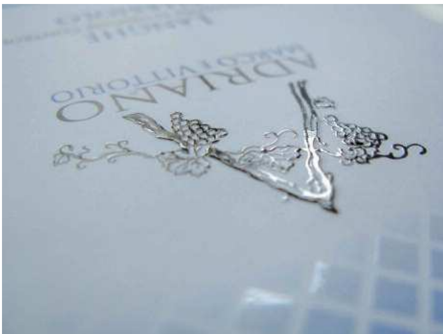
Tactile varnish on pre-printed offset (rotary screen on Gallus)
