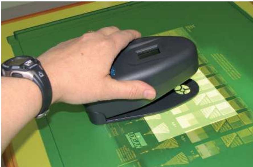
This is the ScreenReader being used to measure the stencil – these values will then be entered in the RIP to linearise the stencil
