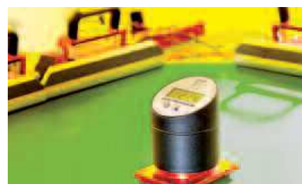
PCF fully coated with the Tensocheck 100 tension measuring instrument
