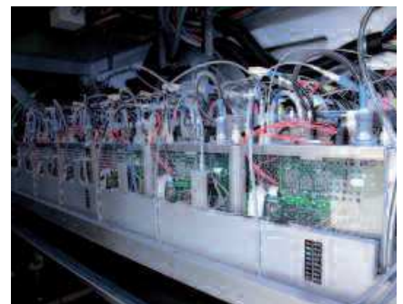
True output speeds of 500 sqm/hr are delivered by an array of 576 Spectra printheads (73,728 actual inkjet nozzles)
