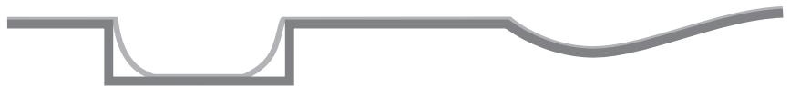
Film lifting due to excess stress – a typical graphic failure in deep corrugations
