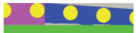
... or else gives negative sawtoothing when the squeegee can't push enough ink through to reach the substrate
