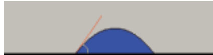
A big ink deposit has a high contact angle and therefore a large slump
