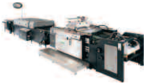
Full in-line integration joins press with feeder, dryer and stacker to a uniform configuration
