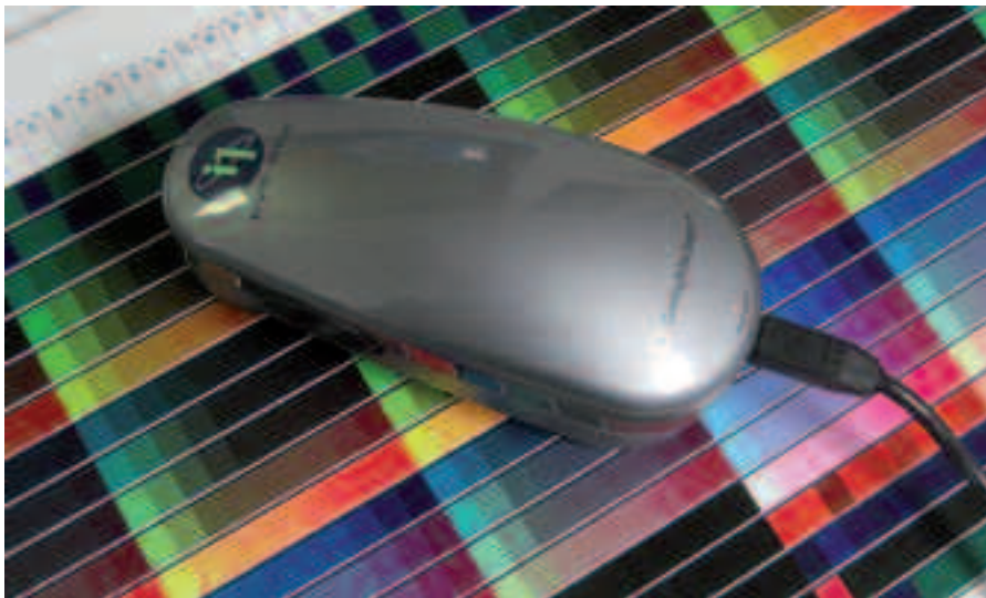
A colour optimiser can be used to manually scan colour targets and to calibrate colour for tools such as computer monitors
