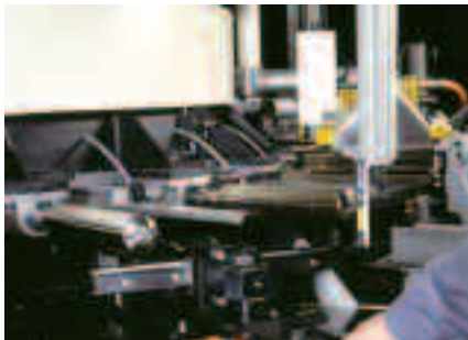
Figure 1: Adjusting the excenter drive of a screen printing machine with rotary indexing table
