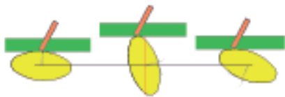
Figure 2: Printing a wrap-around onto an oval container; the diagram illustrates the required movements of squeegee, screen and container
