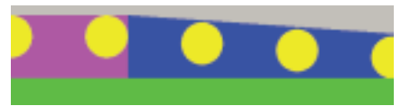
A thick stencil (high EOM) gives a thick edge to the line ...
