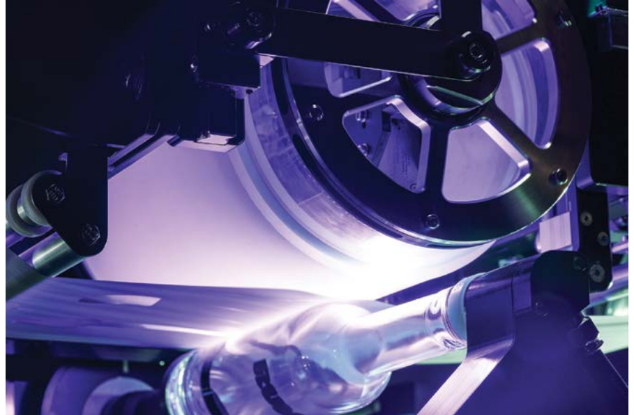
UV LED offers significant advantages over traditional UV curing for screen printing. Photo courtesy of Isimat
