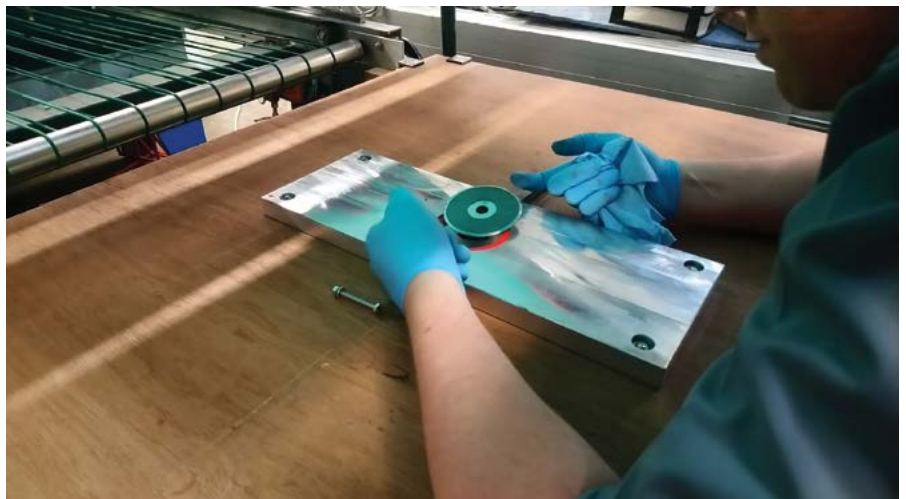
Figure 2: Printing jig being used with a wedge extraction tool
