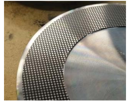
Figure 6: Steel disc printed with etch resist ink
