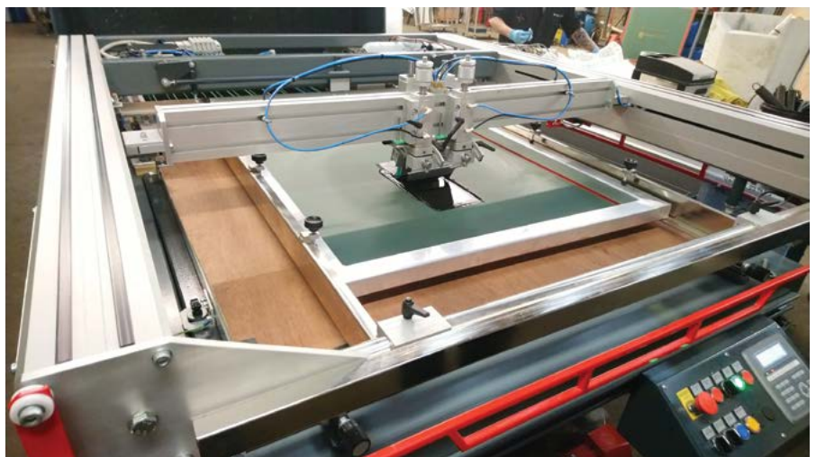
Figure 3: Semi-automatic screen printing machine printing steel discs
