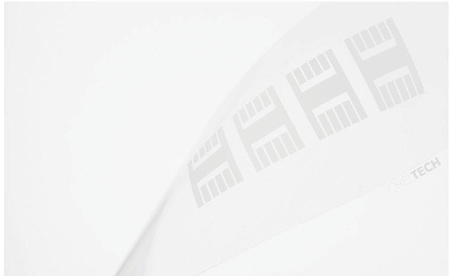
Transparent silver electrode inkjet printed on PET. A working prototype of such an electrode outperformed a reference ITO-based OLED device (M. Hengge et al, Flex. Print. Electron. 6 (2021) 015009). Image reproduced with permission from OrelTech
