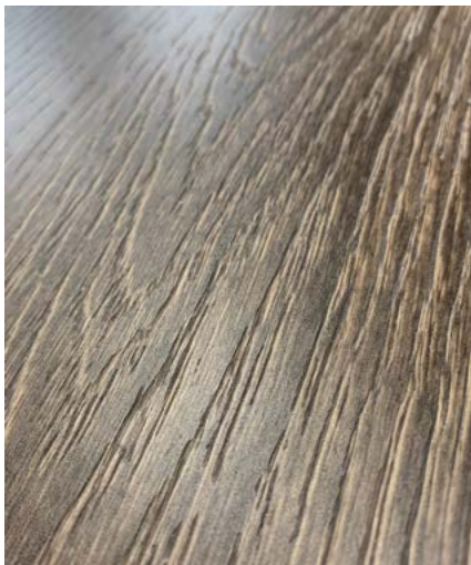
Hymmen's advanced Digital Lacquer Embossing process for floors and furniture offers surface textures with deeper lines and sharp edges
