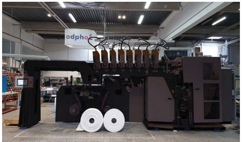
Figure 4: adphos' patent-pending inkjet print production system for narrow flexible packaging and label applications
