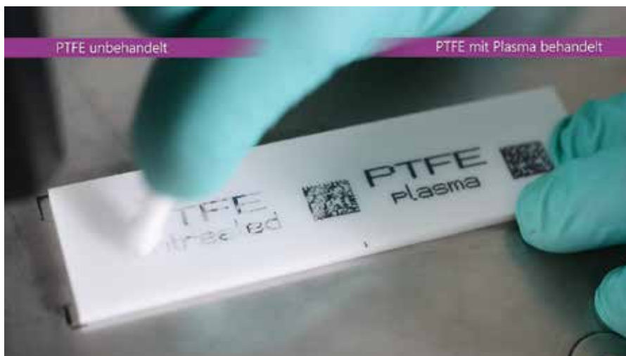
Figure 6: Printing on PTFE (left side untreated and right side plasma-treated)
