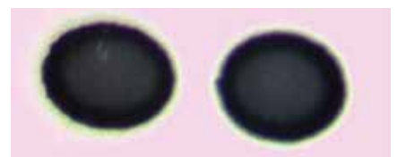
Figure 8: Inkjet printing on high density polyethylene ducts after plasma treatment
