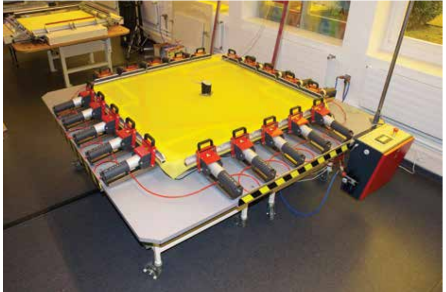
Pneumatic tensioning system, consisting of Sefar 3A clamps combined with Sefar's 51i control unit and Tensocheck 100 tension gauge
