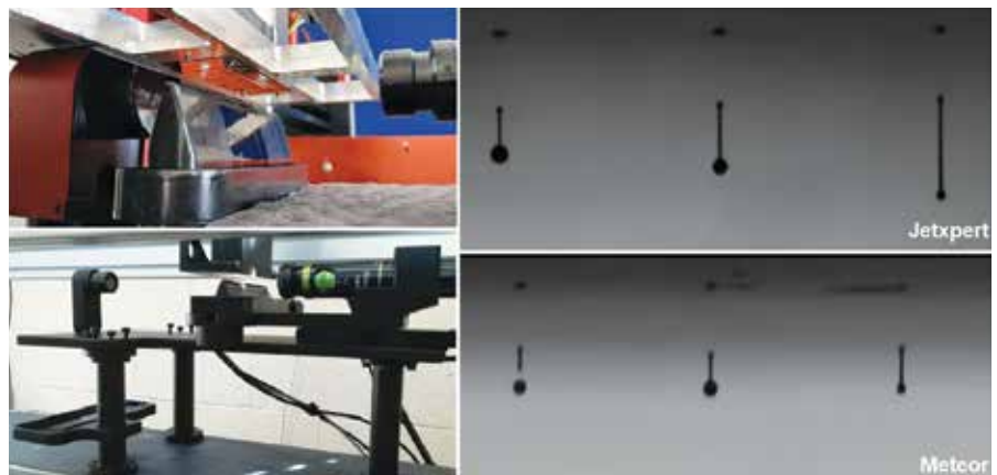
Dropwatchers in DoDxAct's UK lab and example images from looking at a Dimatix SG1024SA printhead
