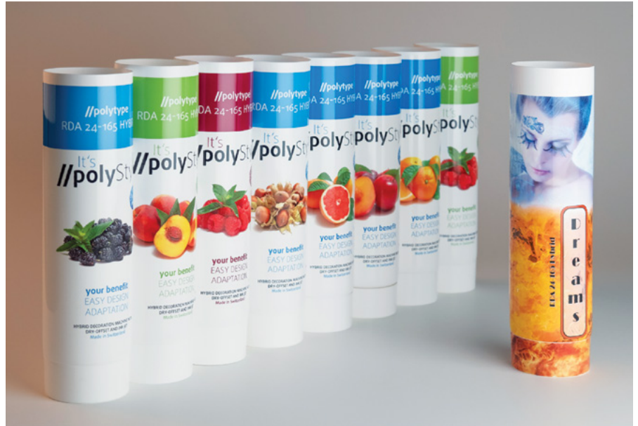
Digitally printed tubes produced on a Polytype DigiTube press using Siegwerk migration-optimised UV inkjet inks
