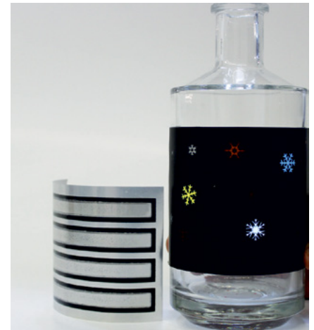
Figure 1: OLEDs powered by a thin and flexible printed battery for a bottle label
