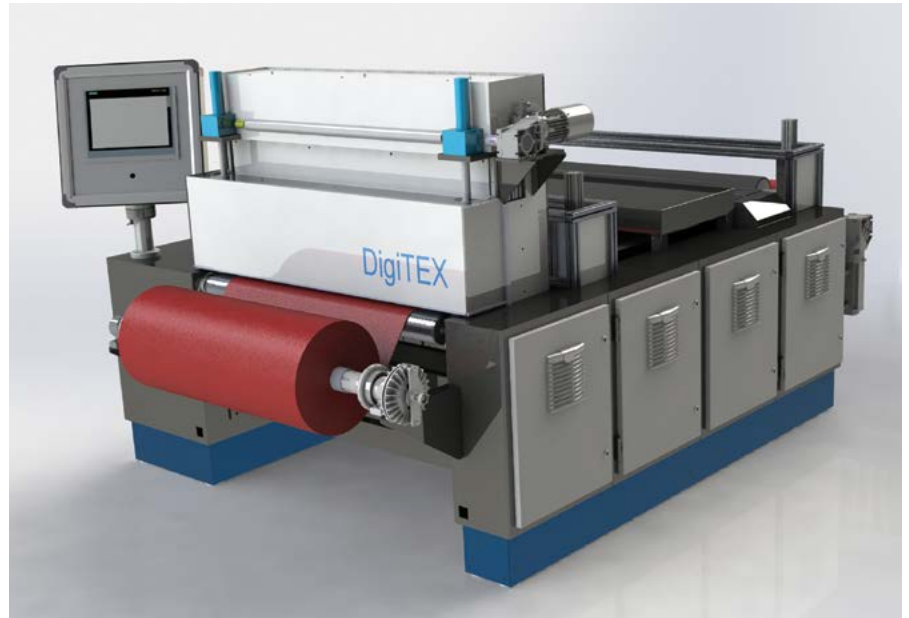
Digital printing machine for textile treatment. The DigiTEXpro project will last until the third quarter of 2021
